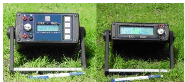
Fig. 8. Electric exploration meter ERA-MAX
